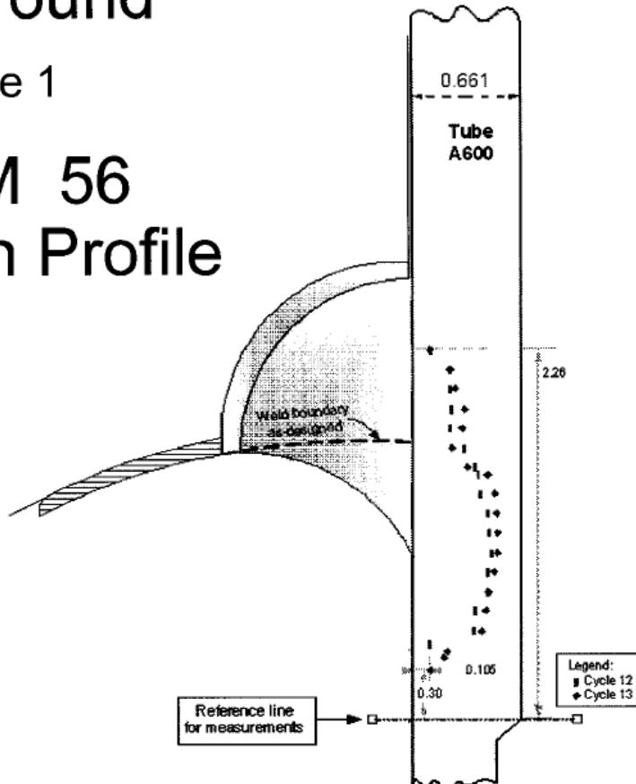
SCE reacted to the signs of crack growth by implementing an NRC-approved repair to CEDM 56. They welded an overlay around CEDM 56 so that the nozzle would remain structurally intact.
